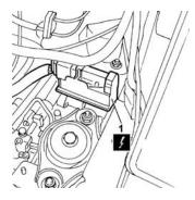
1. Move the front wiring section away from the work area.
