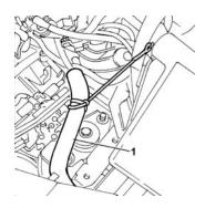
1. Open the retaining band (1a) and disconnect the pipe (1b), tank side.
