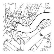
1. Disconnect the electrical connection for the braking system control unit.
