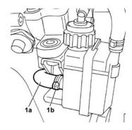
1. Open the band (1a) and disconnect the pipe (1b), electrohydraulic gear selection pump side.
